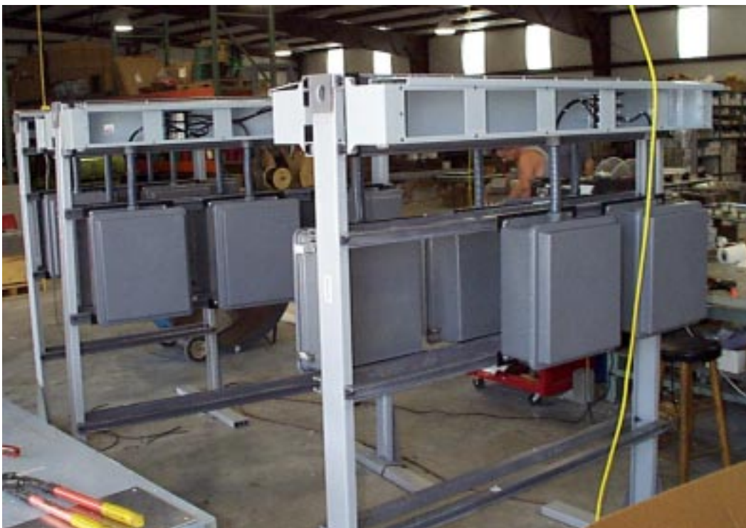
NEMA 4X switchrack. Note that all external devices except for fastening hardware is fiberglass.
