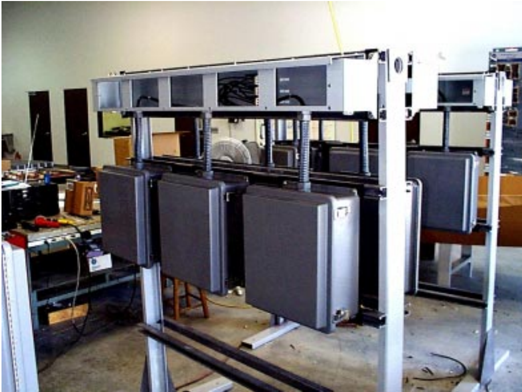
NEMA 4X switchrack. Note that all external devices except for fastening hardware is fiberglass.
