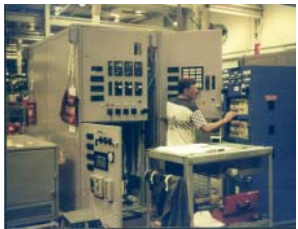
A primary dielectric test of a fully assembled line-up is conducted prior to shipment in accordance with ANSI standards.
