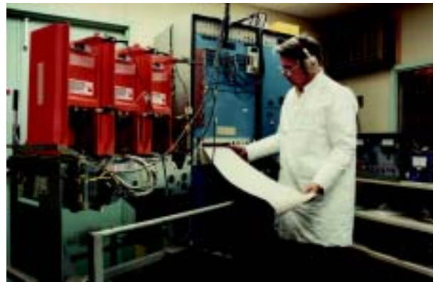
Final breaker test verifies the opening and closing characteristics of every unit.
