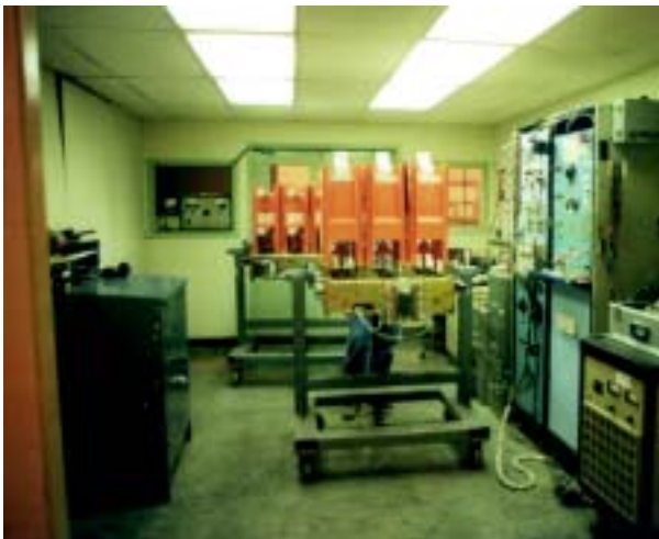
A hi-pot insulation resistance and ohmic test is also performed on every breaker prior to shipment.
